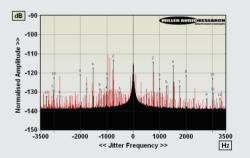
ABOVE: 48kHz/24-bit jitter spectra from AQ DragonFly (via HiFi Rose RS130, black w/mkrs; via PC, red)
