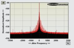
ABOVE: 48kHz/24-bit jitter spectra from iFi Audio's NEO iDSD DAC (via HiFi Rose RS130, black; and PC, red)
