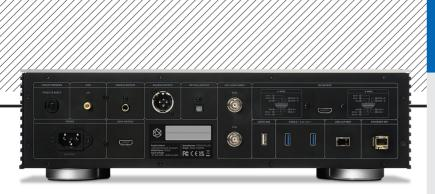
ABOVE: The RS130 offers the option of wired and optical USB/Ethernet inputs alongside two USB-A ports for external media (a bay under the chassis accommodates users' own SSD/HDD hardware). Coax, AES and optical outs are joined by I<sup>2</sup>S on HDMI, video on HDMI, and a USB-A output for connection to an external DAC
